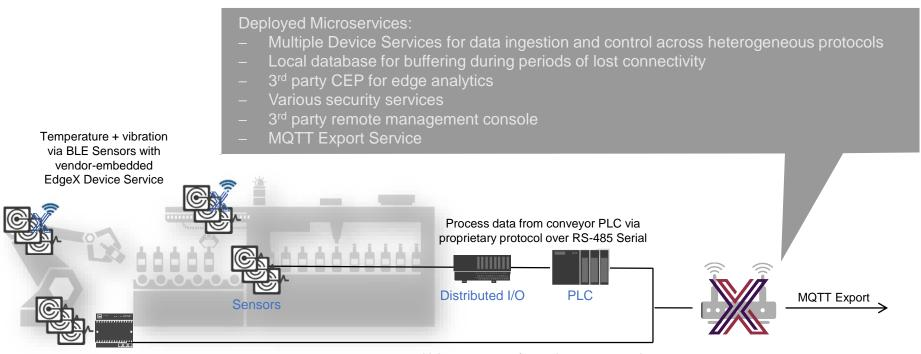
Voltage + current from robot arm motor via power meter, Modbus TCP over Ethernet
