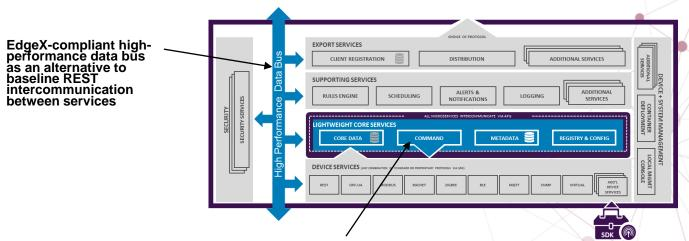
Lightweight, high performance version of Core Services leveraging the key EdgeX APIs at the perimeter. Entire core could even be compressed to a proprietary C-based binary and still benefit from plug-in EdgeX-compliant services from the community.
