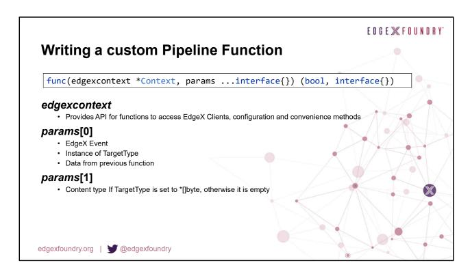
Custom Pipeline functions must to adhere to the AppFunction function signature seen here.
