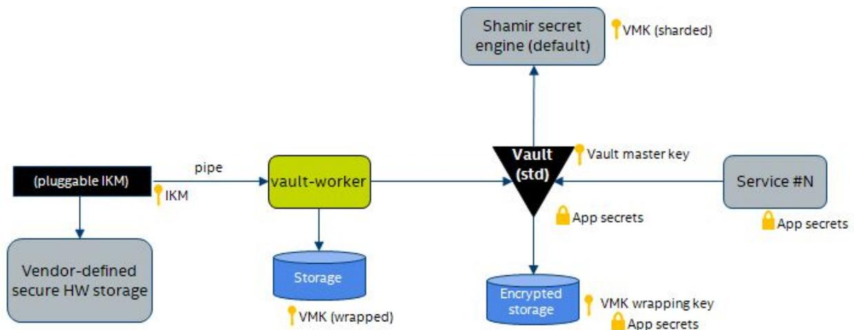
To further strengthen the solution, an implementation can choose to engineer a solution whereby the IKM is only released a configurable number of times per boot, so that malware that runs on the system post-boot cannot retrieve it:
