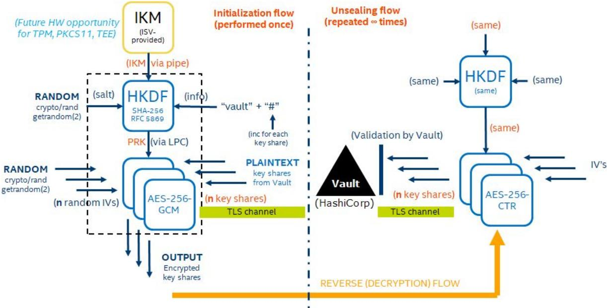
An [RFC-5869](#) KDF requires three inputs. A change to any input results in a different output key:
