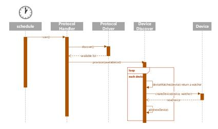
The device SDK code would iterate through the scan results looking for new devices. If a new device was detected, then the SDK would attempt to match the device against any existing ProvisionWatcher objects associated with the
