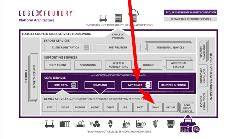
In other cases, automatic discovery of sensors and devices from within EdgeX (typically by a device service) will cause EdgeX to provision a new device. This is referred to as bottom-up provisioning. For example, a BLE device service could be searching for new BLE devices that enter platforms BLE range. If a new sensor is detected in its spectrum, the device service can start to automatically provision that device.
