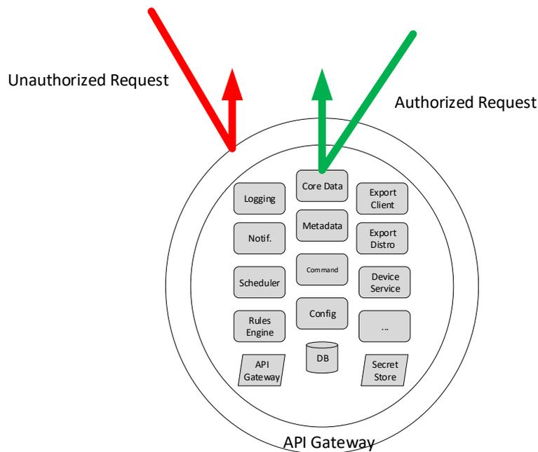
The system management service will assist in protecting EdgeX and reducing the surface area of an API attack. Rather than opening up access to all services to the central management system, the system management service serves as a single point proxy to the control plane for all of EdgeX services for the central management system. The system management system thereby reduces the number of access points to EdgeX and reduces potential security vulnerabilities.
