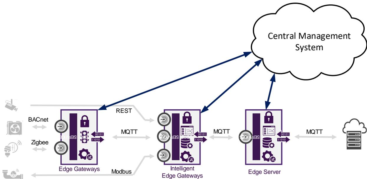
EdgeX system management is not the larger control management system. Instead, EdgeX system management capability is meant to facilitate the larger control management systems. When a management system wants to start or stop the entire fog deployment, EdgeX system management capability is there to receive the command and start or stop the EdgeX platform and associated infrastructure of the EdgeX instance that it is aware of.
