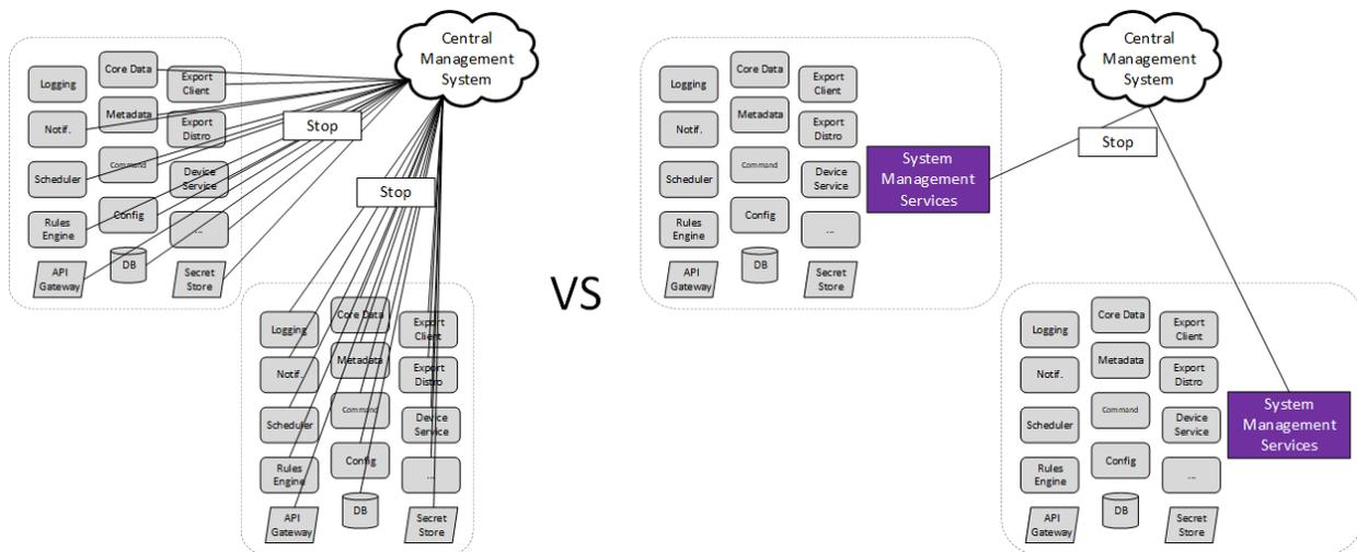
Standardizing operational APIs and making use of an EdgeX control plane service to locally invoke the operational controls potentially reduces remote calls, improves latency, and allows for the operations to cascade from a central management point through a hierarchy of control plane nodes.
