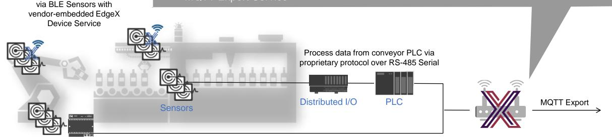
Voltage + current from robot arm motor via power meter, Modbus TCP over Ethernet
