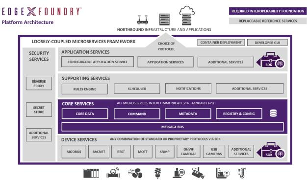
SOUTHBOUND DEVICES, SENSORS, CAMERAS AND ACTUATORS
